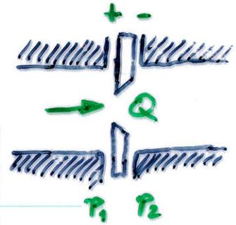
BEI EINEM WIRKDRUCK  $P_1 - P_2 = 4000 \text{ Pa}$  IST EIN VOLUMENSTROM  $Q_V = 1000 \text{ m}^3/\text{h}$  VORHANDEN.
